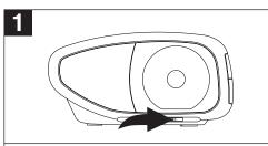
Slide the AUTO/OFF/ON switch to the ON position to turn the unit on; the POWER indicator will light.
